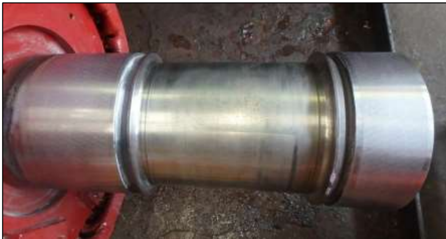
Fig. 25: Condition of rotor shaft journal after repaired by CRC.
