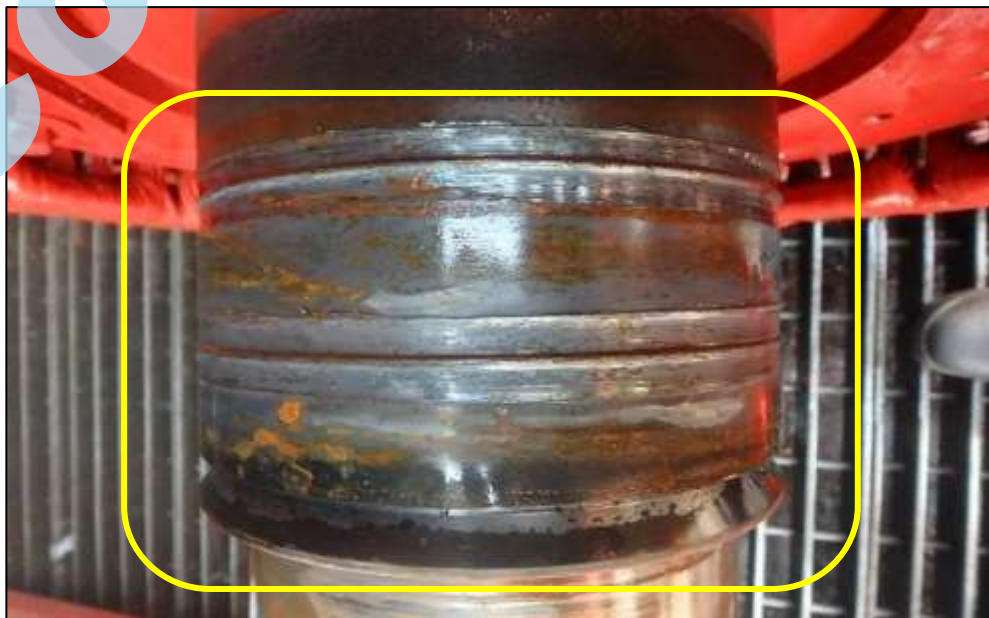
Fig 6 & 7: Condition of rotor shaft journal after dismantling, was found deep score marks. (Shaft journal was repaired by CRC)
