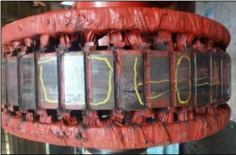
Fig. 8 & 9: Condition of exciter rotor was found with rubbing marks as received.
