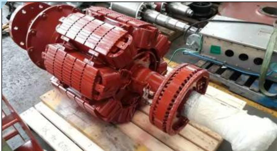
Fig. 19: Condition of Main Rotor after servicing.
