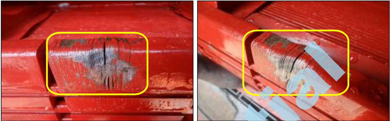
Fig 4 & 5: Condition of main rotor after dismantling, was found dent mark as shown in photo.
