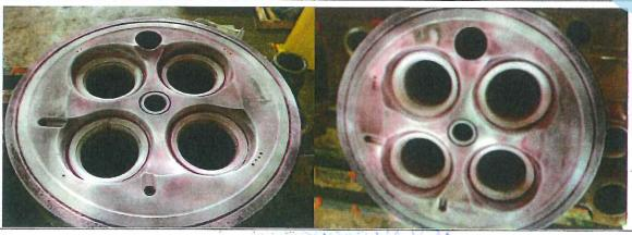
Carried out DVI check on a winder head combustion surface.
